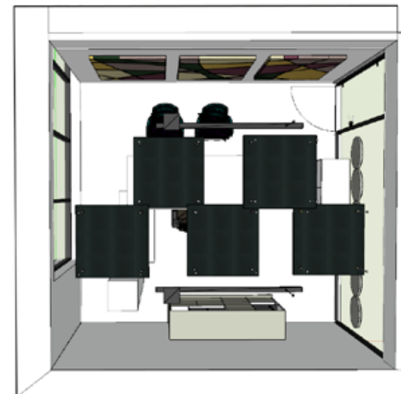
Room after acoustic adaptation - top view
